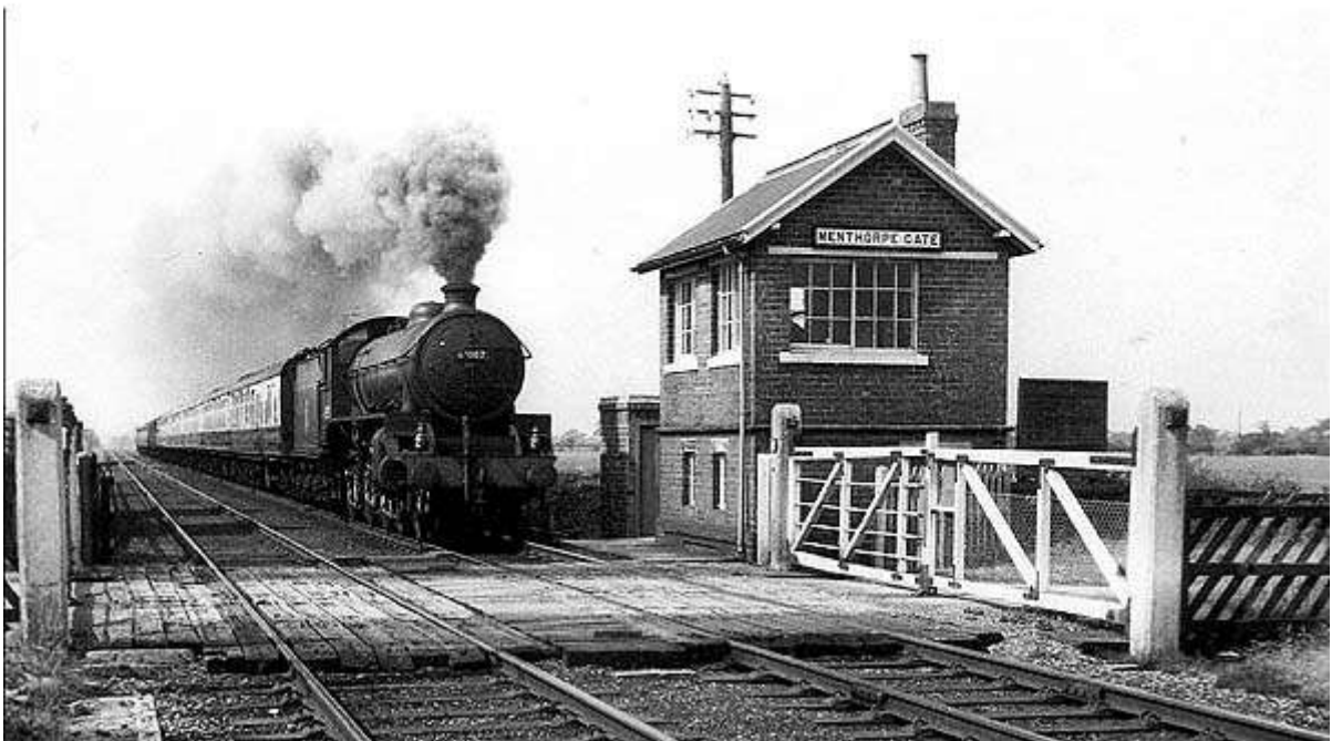
The site of Menthorpe Gate up platform (left) c.late 1950s. The station building was still standing at this time but is out of view to the left. 61087 is an ex-LNER B1 designed by Edward Thompson. Built in 1946 by the North British Locomotive company, Glasgow, it was one of 410 built as a mixed traffic class to rival the LMS Black Five or the GWR Hall. The loco was withdrawn on 5.12.1965 from Doncaster Shed, 36A and cut up in January of 1966 by Garnham, Harris and Elton, Chesterfield. 2 B1s are preserved, 61264 which is now on the NYMR and 61306 which is now named Mayflower.
